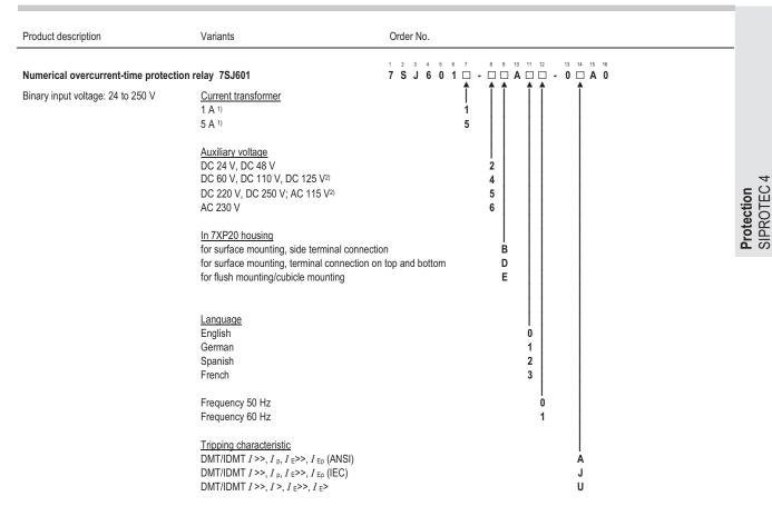
1) Rated current 1/5 A can be selected by means of jumpers.
