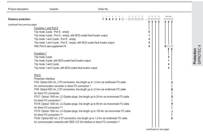
1) Suitable communication converters 7XV5662 (optical to G703.1/X21 or optical to pilot wire) see chapter "Accessories communication"
